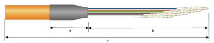
a: 130mm, b: break-out length, could be specified, c: cable length, customer specified
